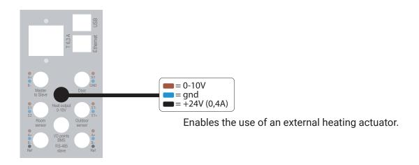
Wiring - I/O Control from Building Automation
